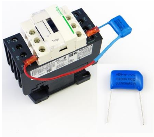
Fig: snubber circuit
